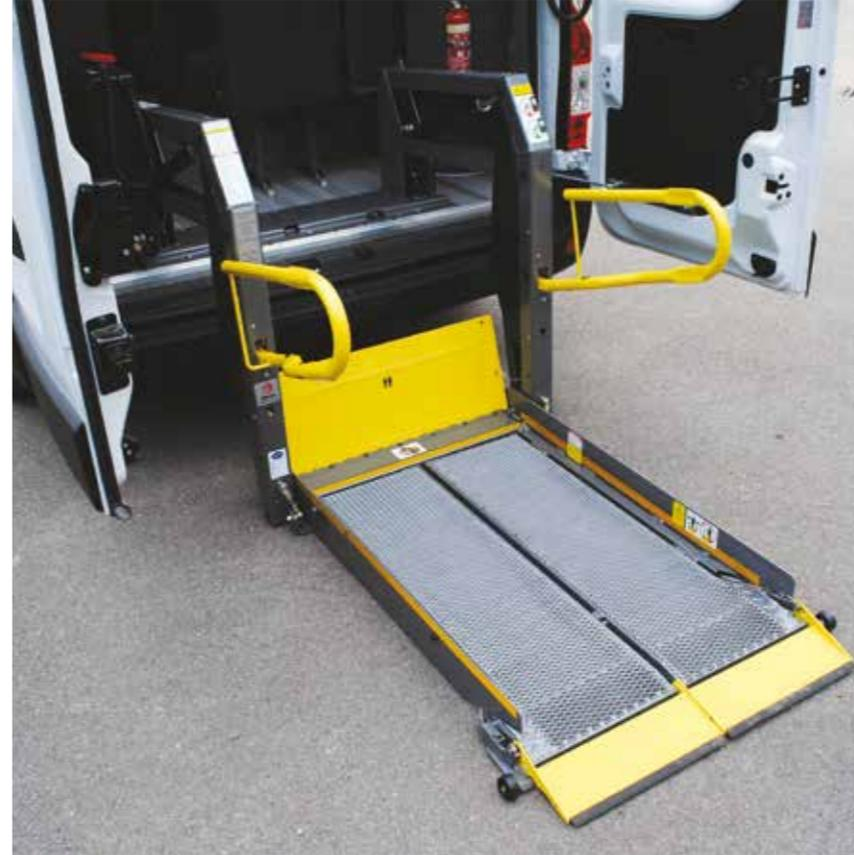
Electric fully automatic stacking tail lift, standard equipment on Wheelchair Access Specification
