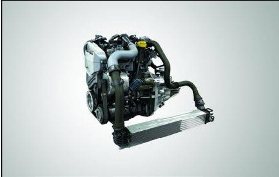
The New Generation Duster RxL Diesel variant with its 1.5 dCi K9K engine will produce **85PS@3750RPM** of maximum power and **200NM@1750RPM** of peak Torque with class leading fuel efficiency of **19.87 Kmpl** which will provide one of the best options for economical city driving with enough power to cruise comfortably on the highway as well.
