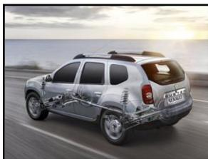
The car is fitted with the all wheel independent multilink suspension for better ride and comfort, regardless of the terrain. Electronic Torque Control (ETC) will ensure intelligent torque distribution to all wheels for high speed high torque balance.
