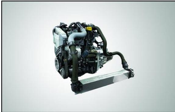
The Renault Duster AWD will be powered by the reliable and fuel efficient 1.5 dCi THP diesel engine (common rail direct injection) delivering a powerful performance with **110PS@4000RPM** of maximum power and peak torque of **245NM@1750RPM**. The engine is mated to a 6 speed manual transmission. This is matched by its excellent fuel efficiency of 19.72 kmpl\*, which is most effective in the eco mode.
