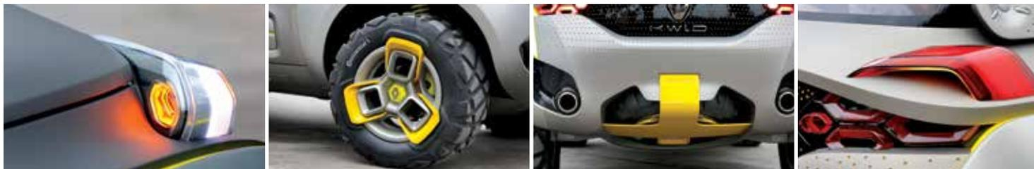
Conceptually cool – hollowed out indicators glow on both sides, specially crafted Continental tyres for show car, spare wheel is slung underneath, unrestrained tail lamps.
