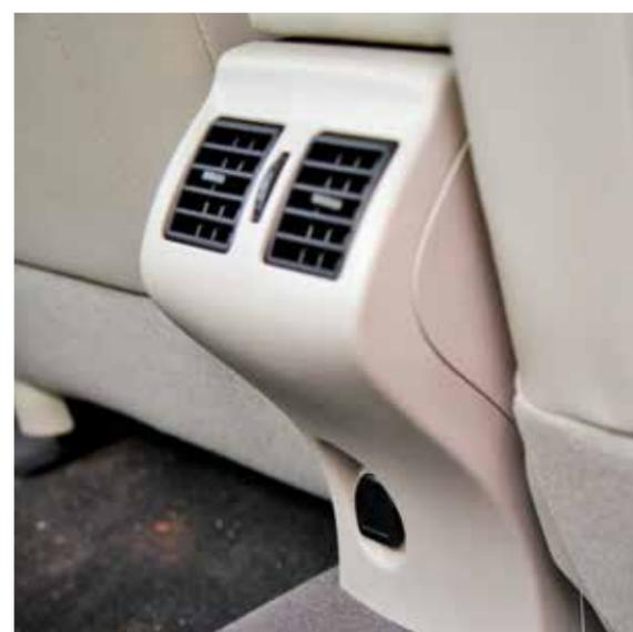
❑ Rear AC vents add comfort for rear passengers. Controller for blower speed would have been nice. Note 12V power socket
